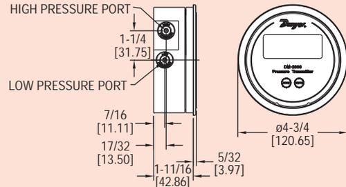
The Dwyer Series DM-2000 Differential Pressure Transmitter senses the pressure of air and compatible gases and sends a standard 4-20 mA output signal. The DM-2000 housing is specifically designed to mount in the same diameter cutout as a standard Magnehelic® gage. A wide range of models are available factory calibrated to specific ranges.
